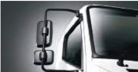
Long stay mirror The long-stay mirrors eliminate the blind spot enabling safer lane changes.
