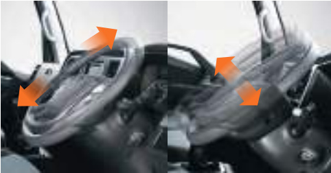
Adjustable steering wheel The tilt angle and distance can easily be adjusted to ensure the perfect driving position.
