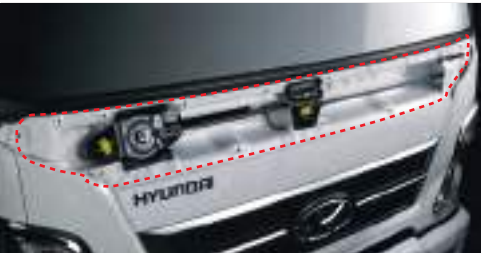
Detachable upper front panel The detachable design allows for quick inspections and easier servicing.
